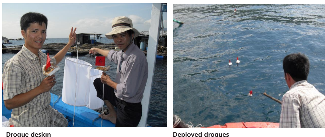
FIGURE 3 Drogues used for the measurement of current dispersion
